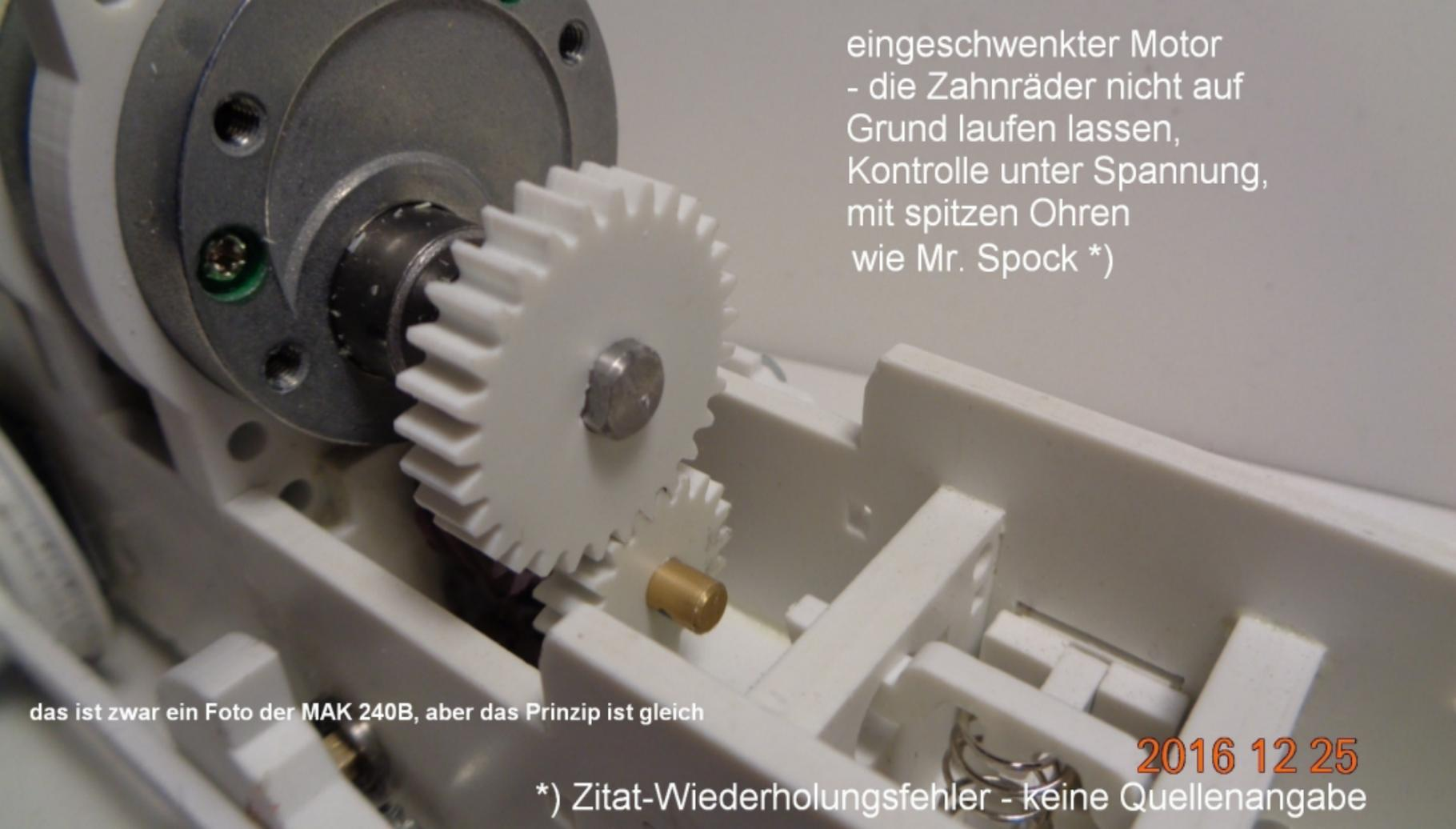
A close-up photograph of a mechanical assembly. A large white gear is mounted on a metal shaft that is part of a motor. The gear is positioned to mesh with a smaller white gear below it. The entire assembly is housed within a white plastic casing. The background is a plain, light-colored surface.
